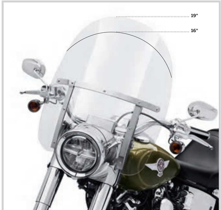
B. KING-SIZE H-D DETACHABLES WINDSHIELD FOR NACELLE-EQUIPPED MODELS WITHOUT AUXILIARY LIGHTING – 19" CLEAR
