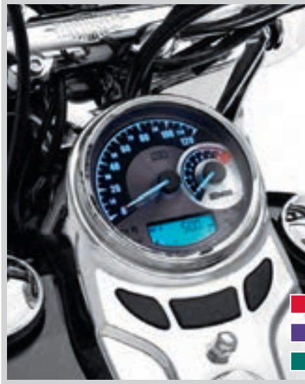
A. COMBINATION ANALOG SPEEDOMETER/TACHOMETER – 5" SPUN ALUMINUM DIAL
