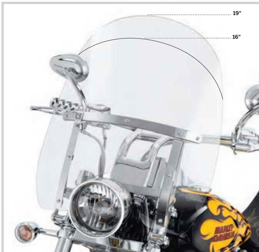
A. QUICK-RELEASE COMPACT WINDSHIELD – POLISHED BRACES (SHOWN WITH TURN SIGNAL RELOCATION KIT)
